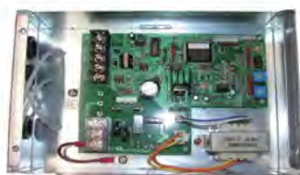
Modbus® Interface TCB-IFMB641TLE
