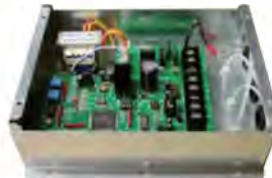
Relay Interface BMS-IFLSV4E For TCS-NET (Max. 64 FCU/Unit)
